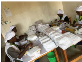
8. Front & back sheets applied and quality control check
